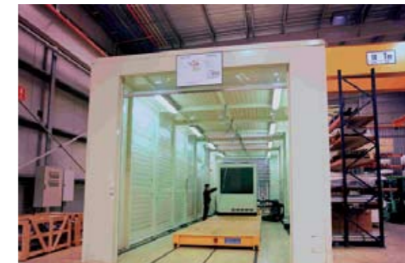
All the chillers are submitted to a Commercial Test, during which the unit is tested by simulating actual operating conditions.
